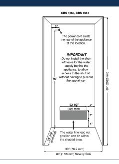
The appliance can be used freestanding or semi built-in. If semi built-in, consider the cabinet opening dimensions.
