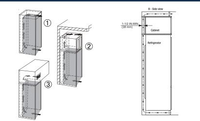
Do not restrict the air flow. The opening can either be directly over the appliance (1), above the cabinet and below the ceiling (2) or through a vent installed in a soffit (3).
