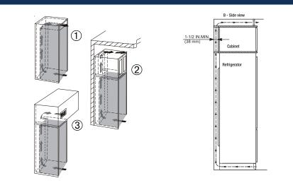
Do not restrict the air flow. The opening can either be directly over the appliance (1), above the cabinet and below the ceiling ② or through a vent installed in a soffit ③.
