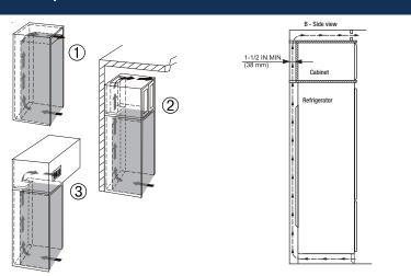
Do not restrict the air flow. The opening can either be directly over the appliance 1, above the cabinet and below the ceiling 2 or through a vent installed in a soffit 3.
