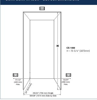
The appliance can be used freestanding or semi built-in. If semi built-in, consider the cabinet opening dimensions.
