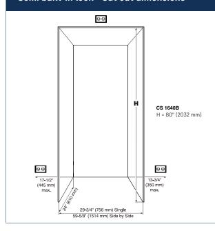
The appliance can be used freestanding or semi built-in. If semi built-in, consider the cabinet opening dimensions.
