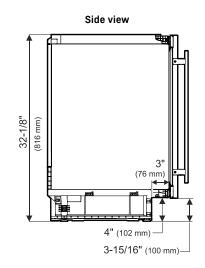
23 - 5/8" (600 mm) min. 24" (610 mm) max. Lim (610 mm) max. Counter depth dimension without cabinet door 28 (578 mm)
