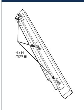
Mount the panel onto the angle bracket using three 4 x 14 screws.
