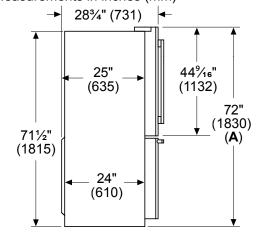
A: Add <sup>5</sup>/8" (17) with front leveling feet fully extended
