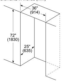
Leave ½" (12.7) gap at the top and 1" (25.4) behind the refrigerator for proper ventilation.
