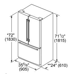
\*Add <sup>5</sup>/8" (17) with front leveling feet fully extended
