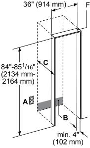
A: Area for installation of power connection.
