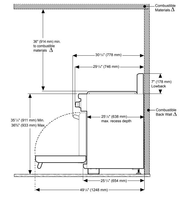
$\Delta$  As defined in the "National Fuel Gas Code" (ANSI Z223.1, Current Edition). Clearances from non-combustible materials are not part of the ANSI Z21.1 scope and are not certified by CSA. Clearances of less than 6" (152 mm) must be approved by the local codes and/or by the local authority having jurisdiction.
