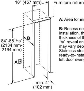
A: Area for installation of power connection.
