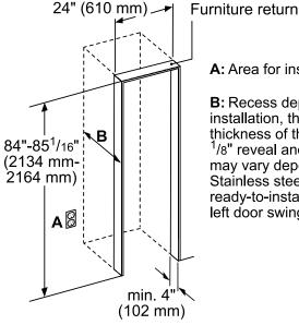
A: Area for installation of power connection.
