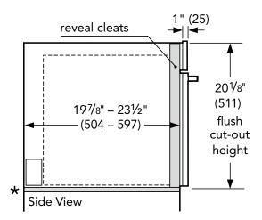
**NOTE:** \* Flush installation requires a 5/16" (8 mm) high x  $28\frac{1}{2}$ " (724 mm) wide x  $22\frac{1}{2}$ " (571 mm) deep baseplate underneath the unit body.
