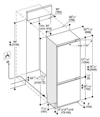
The door face dimensions are designed for a maximum gap of  $\mbox{\em 18}"$  (3 mm).
