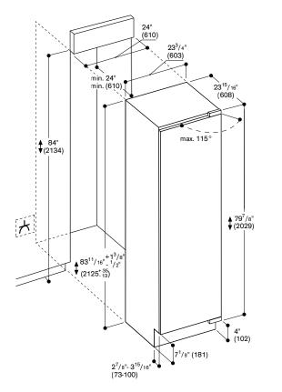
The door face dimensions are designed for a maximum gap of  $1\!\!/\!\!\mathfrak{s}"$  (3 mm).
