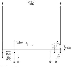
A: LAN connection B: Electric terminal box C: Water outlet D: Cold water inlet
