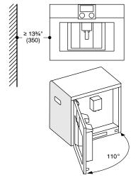
If using the 92  $^\circ$  door hinge restrictor (spare part no. 00636455), the minimum distance from the wall is only 4" (100).
