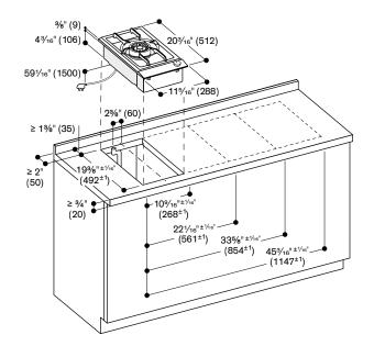
Minimum distance from the appliance cut-out to the side wall  $11^{13}/_{16}$ " (300 mm).
