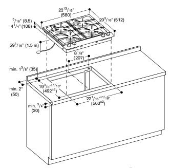
Minimum distance from the appliance cut-out to the side wall 11<sup>13</sup>/16" (300 mm).
