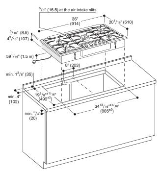
Minimum distance from the appliance cut-out to the side wall 11<sup>13</sup>/16" (300 mm).
