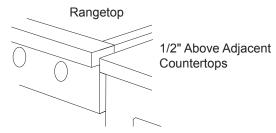
Front of deep cabinets can align with control panel beveled edge.
