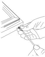
• Insert the new bottom plug/bushing in the new bottom of the door. Secure with the screw removed from the old plug/bushing.
