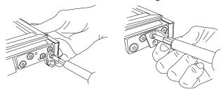
Install the bottom trim onto the new bottom side of the door.
