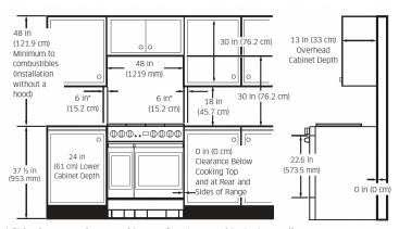
$<sup>^{\</sup>star}$  Side clearance above cooking surface to any objects, i.e., wall.
