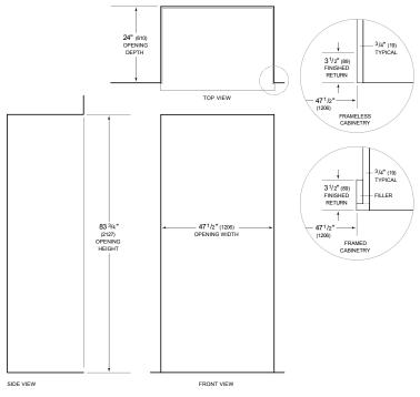
NOTE:  $3^1/2^n$  (89) finished returns will be visible and should be finished to match cabinetry Shaded line represents profile of unit.
