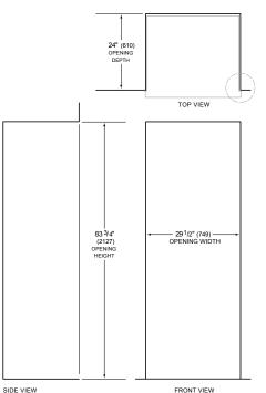
NOTE:  $3^{1/2^{\ast}}(89)$  finished returns will be visible and should be finished to match cabinetry Shaded line represents profile of unit.
