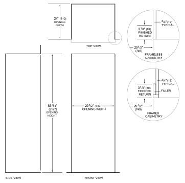
NOTE:  $3^1/2^n$  (89) finished returns will be visible and should be finished to match cabinetry Shaded line represents profile of unit.
