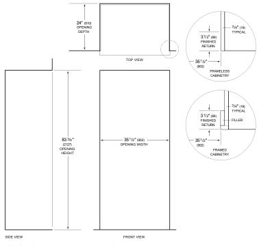
NOTE:  $3^{1/2^{\ast}}(89)$  finished returns will be visible and should be finished to match cabinetry Shaded line represents profile of unit.
