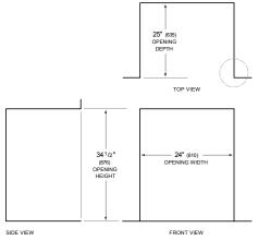
NOTE: 31/2" (89) finished returns will be visible and should be finished to match cabinetry
