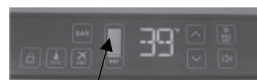
9. After you change the bulb, press the Refrigerator icon and hold for 3 seconds. The icon will turn white which means the bulb counter has been reset.
